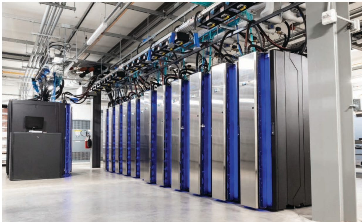
WCOSS supercomputer system: 14.5 PetaFLOPS (Recall ENIAC = 40 OPS: 15 orders of magnitude in 80 years!)
